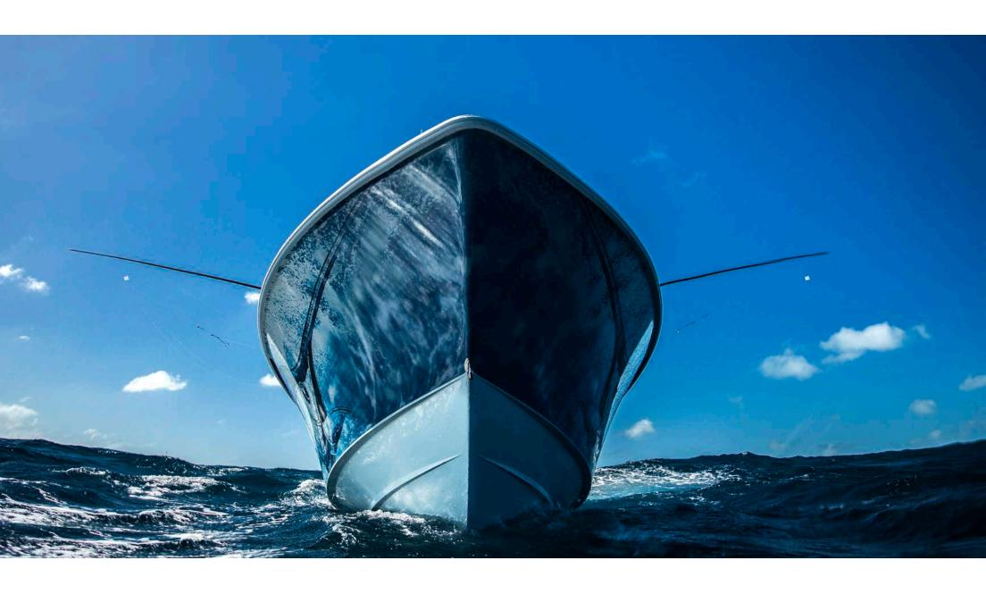
Every Contender is built with hand laid fiberglass using multi-directional fabric and foam cored solid glass stringer system. The hull is laminated solid fiberglass using biaxial and triaxial cloths, structural PVC core sandwich construction, vinylester resins and specially formulated gel coats for high gloss mirror like finish.
