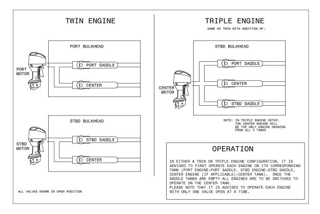
When equipped with three fuel tanks, there will be one fill located on the starboard side (for the starboard saddle tank) and two located on the port side. One of the fills on the port side will have a small "C" etched in it, to signify the center tank.
